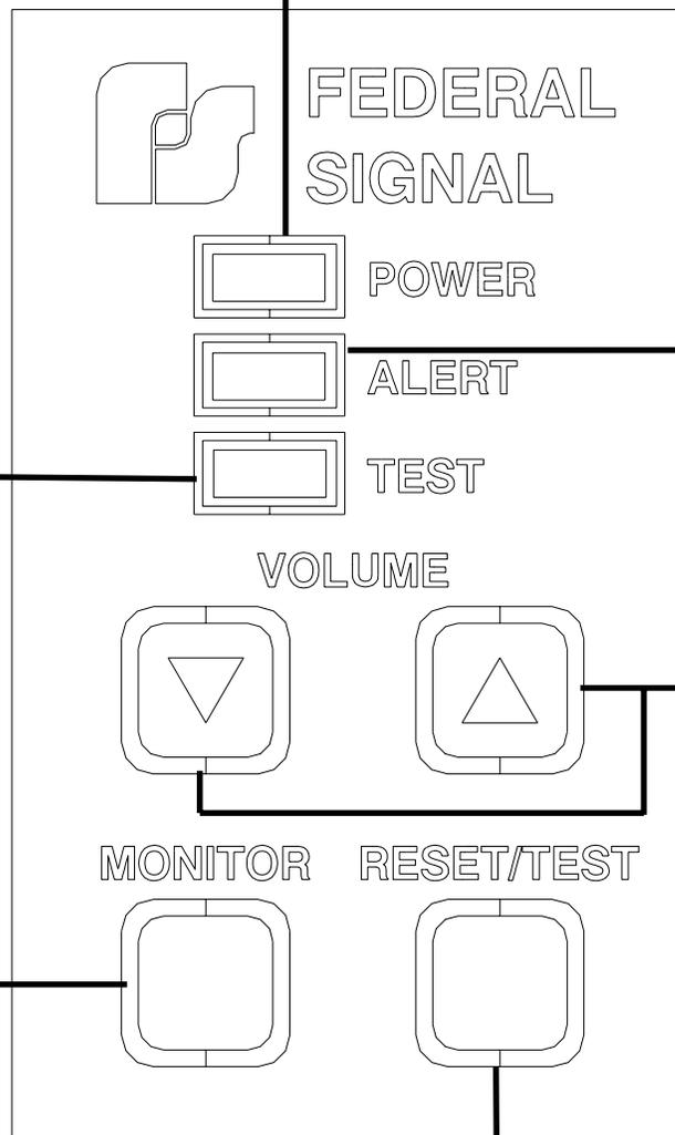
**ALERT LED** flashes Red when TAR receives an Alert Message. The TAR may also give a series of loud beeps and open the channel to provide an alert message. *You should immediately respond as instructed.* The **ALERT LED** will continue to flash until you press the **RESET** button below.
