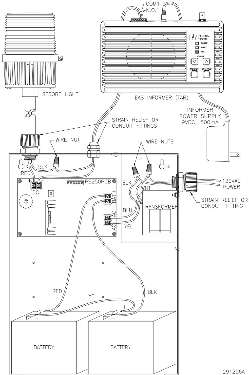
**Model FB2PST-012-024C Strobe Light Accessory Wiring Diagram**
